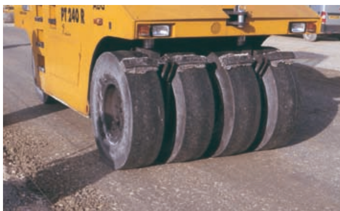
Figure 6: Mixture M7 under pneumatic-tyred roller
